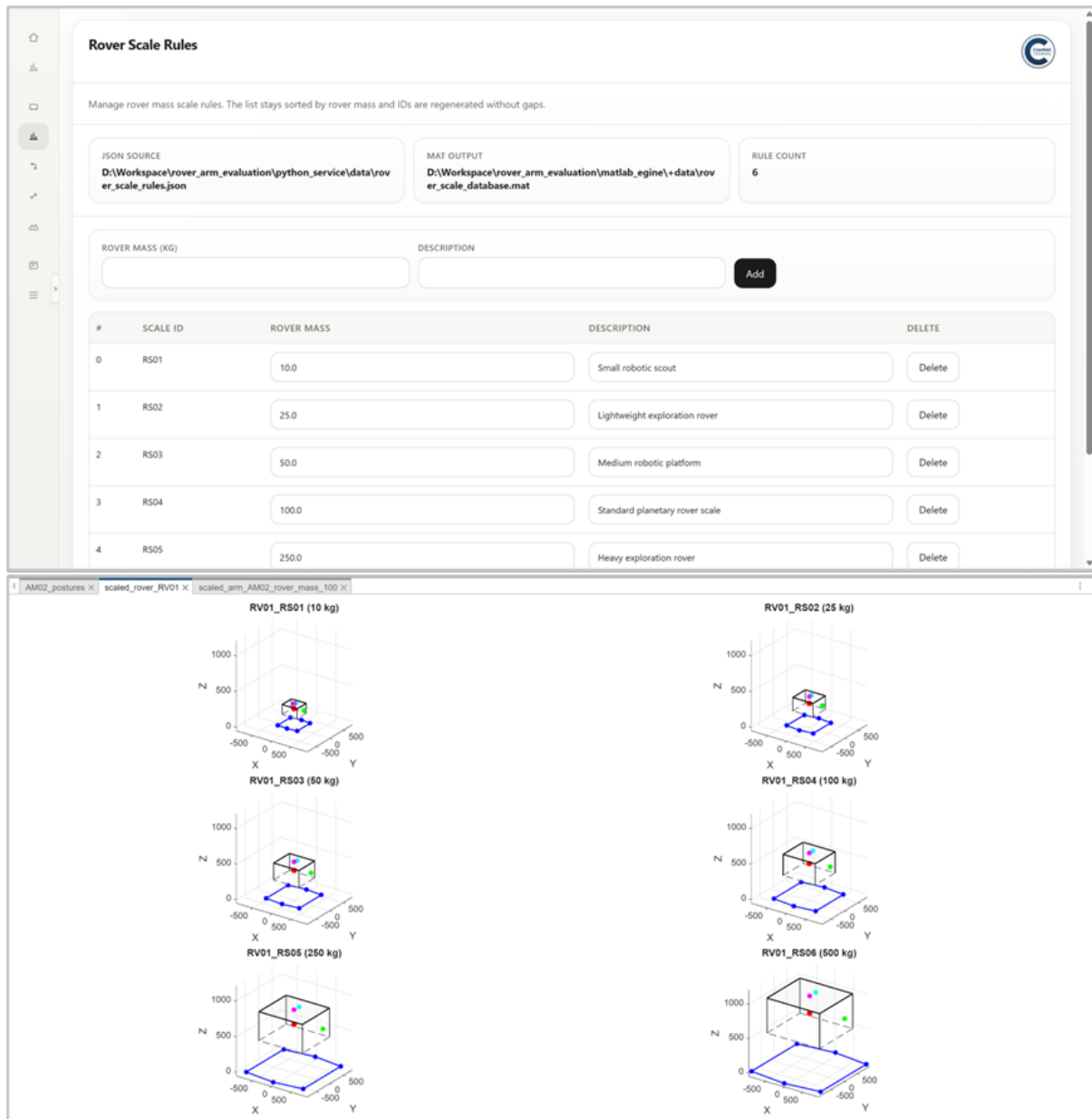
Figure A.8: Rover scaling mechanism and geometric effects. (a) Definition of rover mass scale rules; (b–g) resulting geometric configurations across different scale levels, illustrating variations in support polygon and centre of mass distribution
