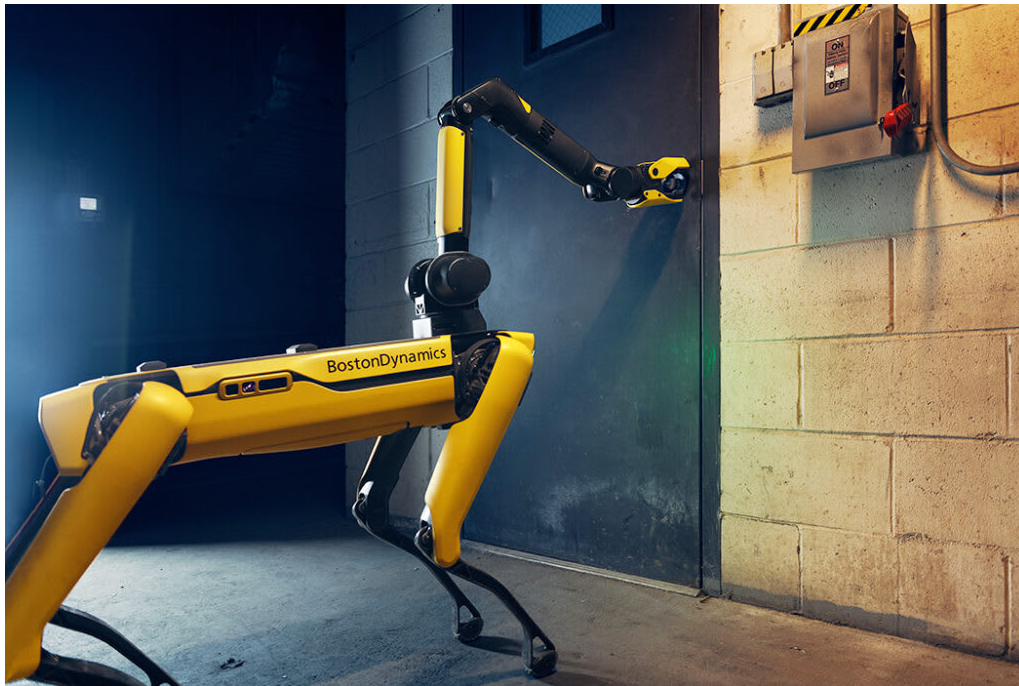
Figure 2.8: Boston Dynamics Spot with the integrated 6-DOF Spot Arm performing a contact manipulation task — the hardware platform deployed in the ReLIC loco-manipulation framework. The front-mounted arm configuration provides a 984 mm reach envelope directly aligned with the robot’s locomotive heading.
