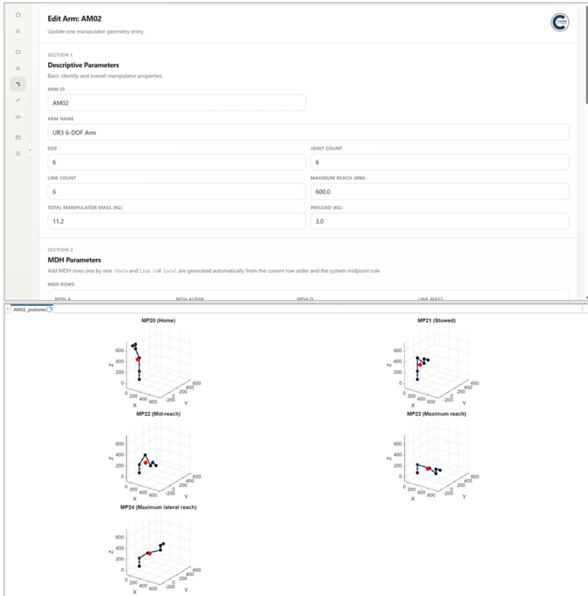
Figure A.7: Manipulator configuration interface and pose visualisations, illustrating multiple predefined arm configurations (e.g., home, stowed, and extended poses) used for reachability and stability evaluation
