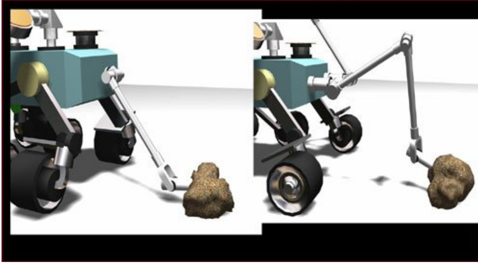
Figure 2.15: Comparison of rover–manipulator coordination strategies: a 2-DOF manipulator utilising base mobility (left) versus a 5-DOF arm operating from a stationary platform (right).
